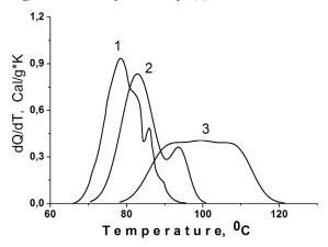
Fig. 2. Heat absorption curves of the DNA-Cu(II)TOEPyP (4) complex at various values of r. 1) DNA without Cu(II) TOEPyP(4); 2) r=0.007; 3) r=0.07
