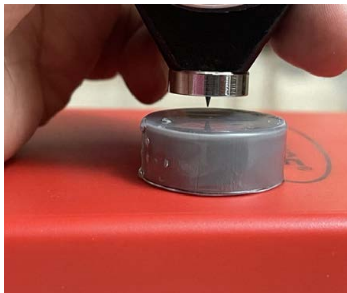
Figure 2. Hardness measurement by using shore D hardness (Shore D hardness tester \ India MART-INDIA 2022).
